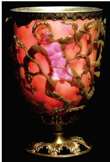
Figure 1. The Lycurgus Cup, an example of nanochemistry under glass from antiquity, where glass serves as a host for functional nanoparticles, e.g., gold colloid. Copyright Trustees of the British Museum.
